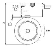
T Distance sensor head / magnetic ring: 0.1 ... 1.5 [0.004 ... 0.06] (1 [0.04] recommended)
