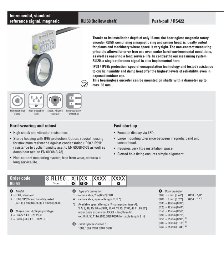
1) Cable lengths >10 m only possible with supply voltage >10 V.
