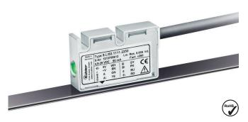
The non-contact incremental magnetic linear measurement system Limes LI50 / B2 - made up of the sensor head LI50 and of the magnetic band B2 - reaches a resolution up to 5 µm with a maximum distance of 2 mm between the sensor and the band.
