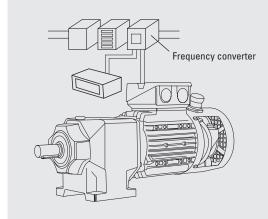
Control of simple, time-based processes by means of an analog signal, e.g. ramping control for locks and sluices
