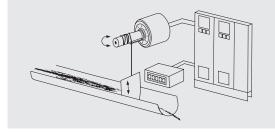
Calibration of filling levels and flow rates: the setpoint adjuster simulates the output signals of a level or flow sensor for configuring a control.
