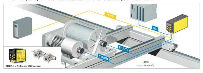
3 - Safe hoist position and winch speed thanks to the certified Profisafe Sendix S58FS3 encoder. The encoder transmits the position of the load and the speed of the winch directly to the safety controller. An incremental encoder, e.g. Sendix 5020, measures the motor speed and transmits it to the inverter. By measuring the speed at the motor and at the rope drum, the drive train can additionally be monitored for mechanical damage such as slippage or gear breakage.
