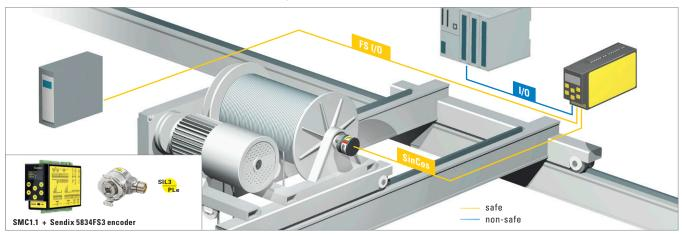
2 - Safe detection of overspeed by an SMC2.4 module with two diversitary incremental encoders, e.g. Sendix 5020. By detecting the speed at the motor and at the wire drum, the drive train can additionally be monitored for mechanical damage such as slip or gear breakage. The safe digital outputs of the SMC module activate the STO function (Safe Torque Off) of the inverter.
